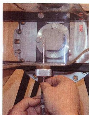
8. Put the plastic clamps (plexi fixtures) on the probe holder (above the shielding tube) and hold them tight (Figure b).
