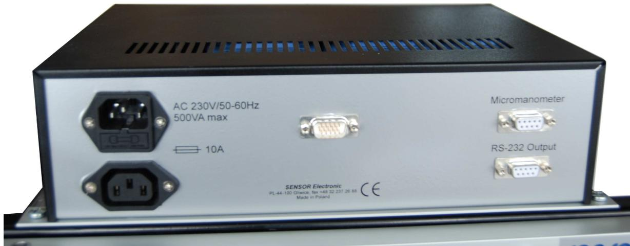
On the back panel, there are: on the right side - socket for connecting a computer port RS232 and socket for connecting a micromanometer; in the centre - socket to connecting the Switch Driver and Air Temperature Sensor; on the left side – sockets for main power supply and fan power supply.
