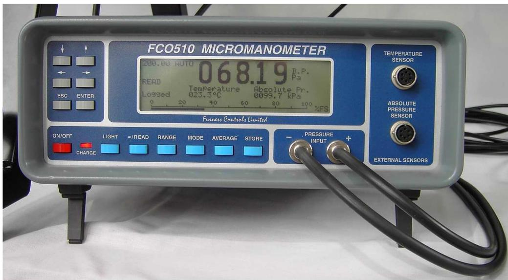
In order that all properties of the tunnel and the software can be exploited the Micromanometer Furness Controls FC0510 of the range 0÷2000 Pa is required to be associated with the tunnel. Using the micromanometer with a serial output RS232 makes it possible to run automatic control of velocity and automatic calibration procedures.
