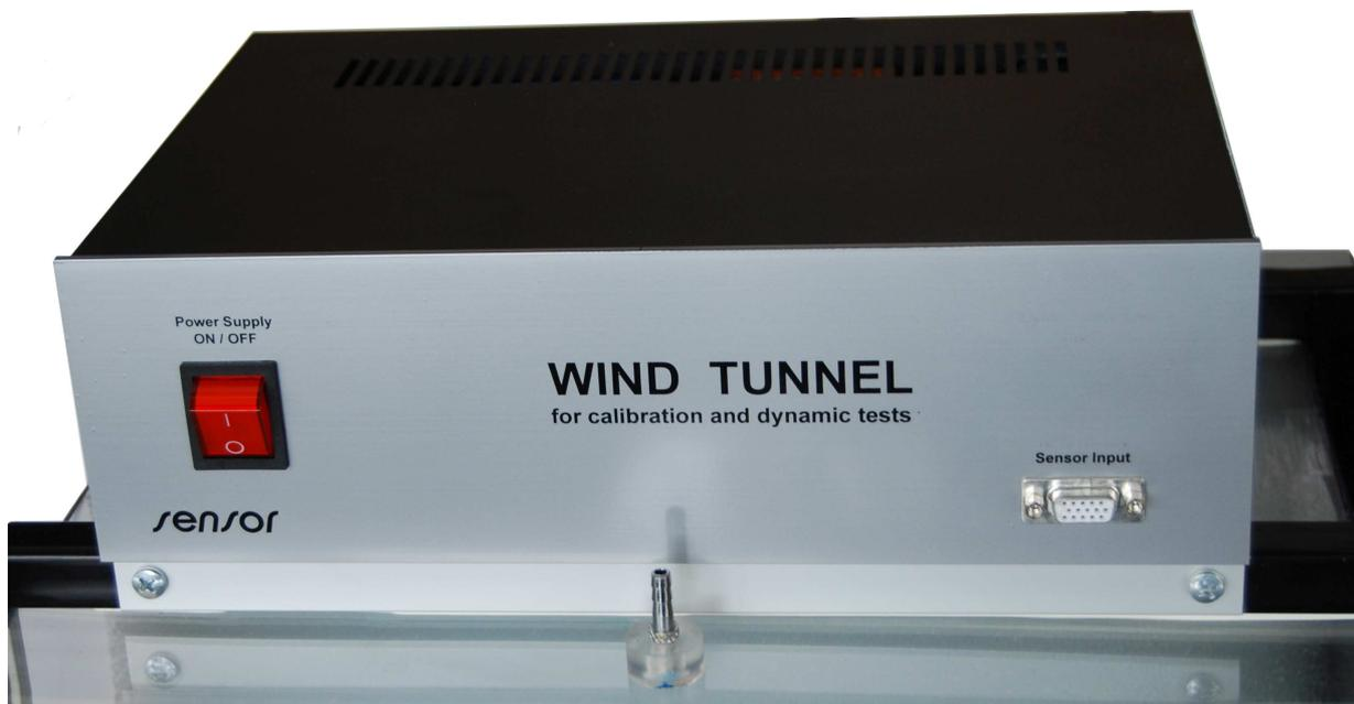
The Control Module contains the elements that are necessary for correct operation of the tunnel. It is comprised of: air temperature unit, barometric pressure unit, A/D converter with two analog differential inputs, serial communication RS232 module and AC/DC adapters.
