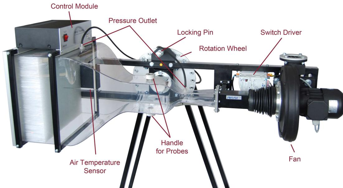
A separate Switch Driver controls a fan used for precise and steady flow generation. The wind tunnel is equipped with a control module which comprises barometric pressure and air temperature measuring units, AD converter with two analog inputs, RS232 interface and power supplies adaptors. An RS232 output enables the computer to control and calculate the flow velocity in the wind tunnel.
